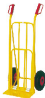
HT1826 (HT1827AN) Weight(kg):11 Load Capacity(kg):180 Pneumatic Tyre:3.00-4 L/W/H(mm):1115x520x470(840)
