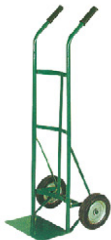
HT1545 Weight(kg):9.6 Load Capacity(kg):150 Solid Tyre:8"x2" L/W/H(mm):1180x470x435
